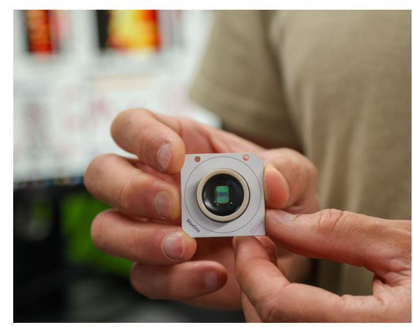
Figure 1. CMOS-based microelectrode array chip. These devices contain thousands of miniaturized amplifiers used to triangulate the electrical activity of single neurons within millimeter-sized organoid tissue (Photo taken by Sharf Lab, UCSC)
